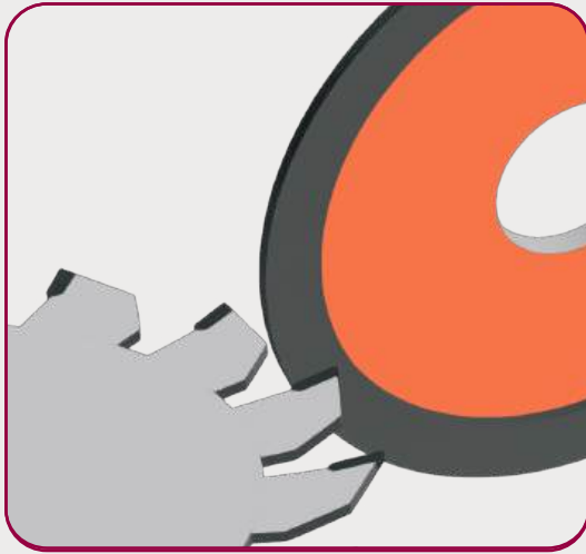
Face grinding of the tool
