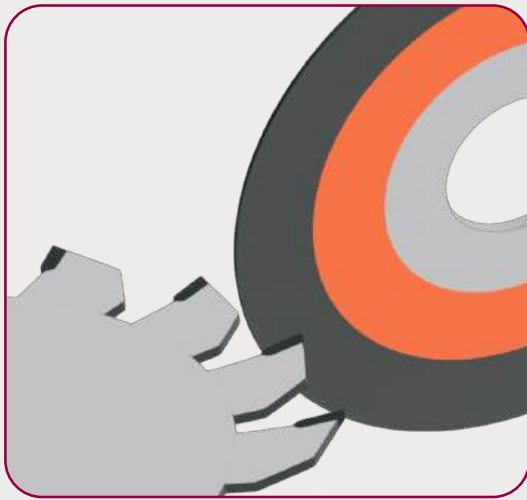
Face grinding of the tool
