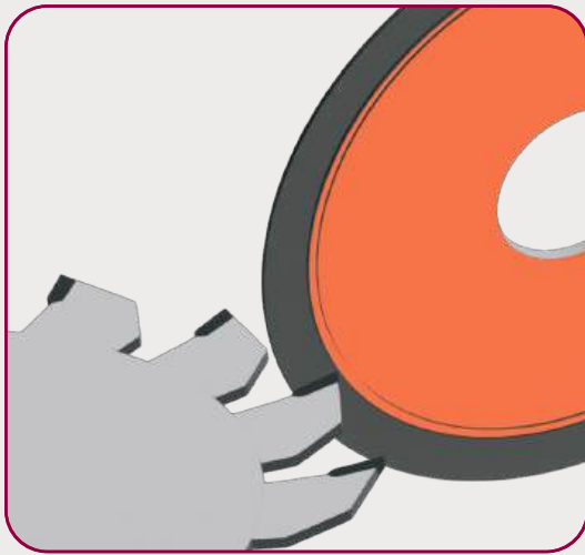
Face grinding of the tool
