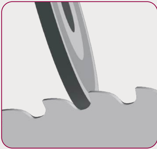
Sharpening and reprofiling of HSS circular saws
